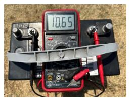
This is NOT what you want to see! At 10.65 Volts, this battery is fully discharged. It didn't recover after being charged. Subsequent testing showed it had no capacity, and is junk.
