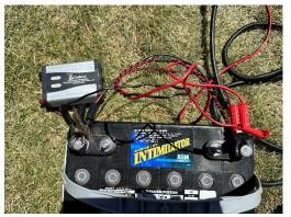
This is the battery with both the solar controller and a small generic inverter clipped on.
