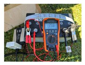
This battery is sitting fully charged at 13.56 Volts. This is the high voltage set point for the regulator in this generic controller.
