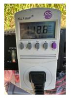
Here's the inverter output voltage (112.6 VAC) with a 1500 watt rated unit delivering 800 watts to a coffee pot (about 7.0 Amps). This is on the low end of the output voltage, but there is quite a bit of sag due to the high current voltage drop in the DC cables going to the inverter (3 SLA's in parallel for 12 Volts at roughly 300 AH capacity).
