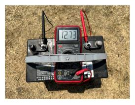
At 12.73 Volts, this battery is essentially fully charged. It's a perfect candidate to be put into service, either by itself or together with several other similar high charge state batteries.
