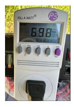
Plug either an outlet strip or heavy duty extension cord into the Kill-A-Watt to distribute power (6.98 Amps AC to power the coffee pot).
