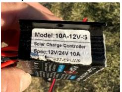
The controller on the left is a generic 12 or 24 Volt automatic unit capable of 10 Amps, with an SLA battery. It's waterproof and simple, and will
