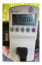
This is reading the real time power delivered to the coffee pot: 785 Watts (112.6 Volts times 6.98 Amps).
