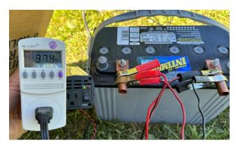
This is a setup using alligator clips and optional terminal extenders with both the solar controller and low power inverter (ca. 400 watts). It's shown delivering 37.4 watts to a soldering iron. That's just a little more than a CPAP machine uses with the heater tube turned on in cold weather.
